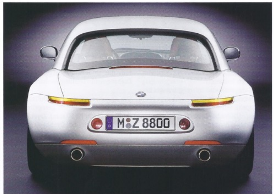
Figure 24: Rear light units with direction indicators, reversing and brake lights in neon technology. Rear fog light and reversing lights
