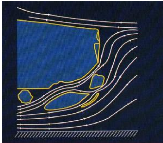
Air flow pattern around the Z1 rear exhaust box and body panels
